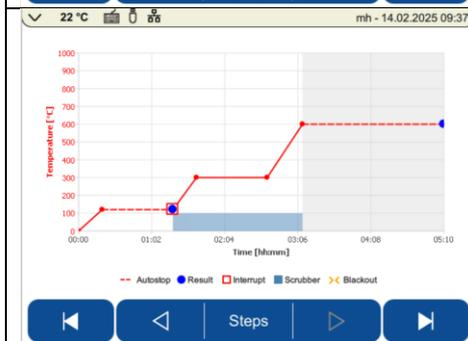
The use of the scrubber is necessary in all steps in which acid vapors are produced, namely when fuming off the sulfuric acid during the sulfated ash determination.
