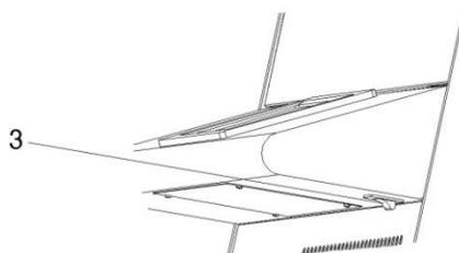
**3** The main switch (3) is located on the underside of the console.
