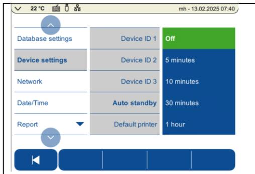
Specify whether and when prepASH switches to standby mode. If the user has a password, this must be entered again to exit standby mode. If the device switches to standby mode during the analysis, the measurement is continued immediately. (see also 6.7 Standby activated/User password)
