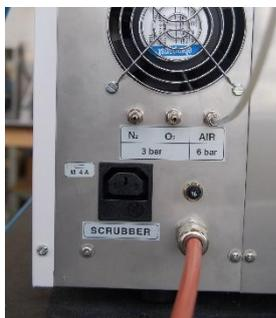
Connect the scrubber to the mains socket on the back of the prepASH. Use the special mains cable from the scrubber connection set 340-9002.
