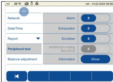
You can control and test the scrubber in the Periphery test (settings). If you set the controller to “on”, the pump should be audible and the wash water should bubble.
