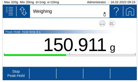
(After the hold time has run out. the peak-hold is cleared and the display shows the current weight on the pan again.)
