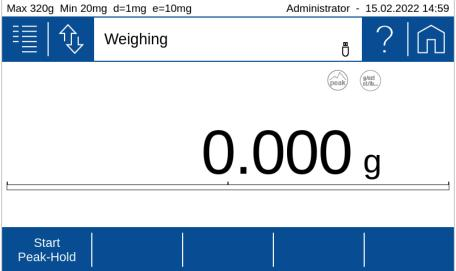
Place the weight on the weighing pan. The maximum measured **stable** weight value is displayed and held until **[Stop Peak-Hold]** is pressed.
