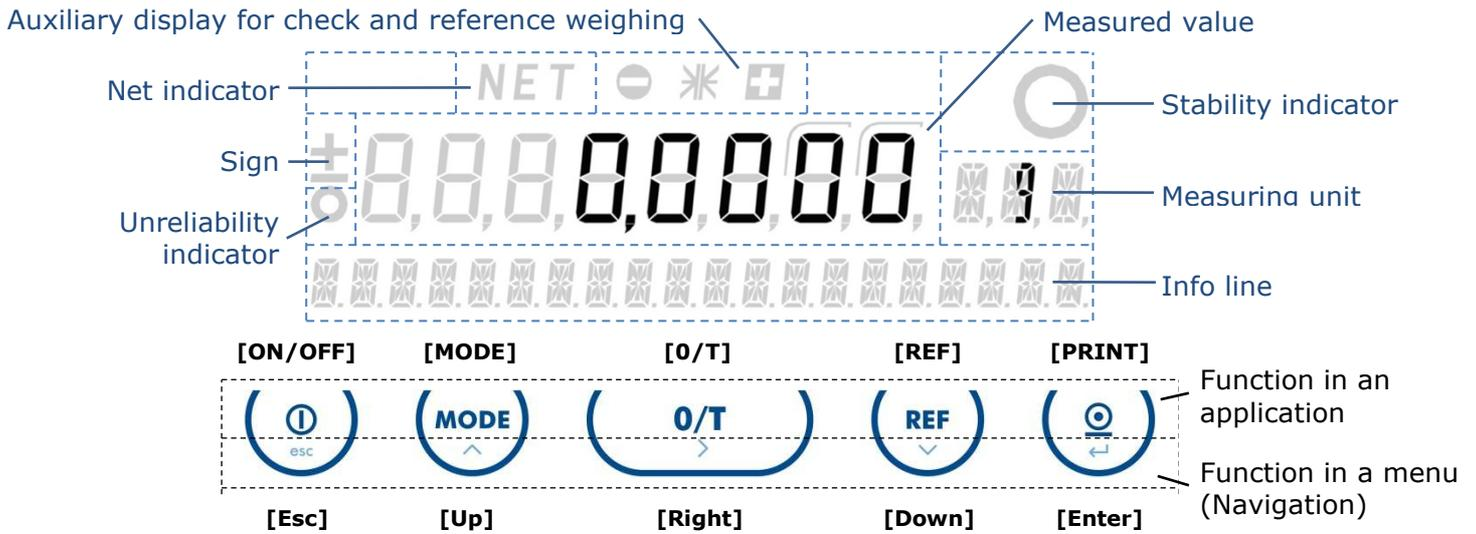
The measured value is stable as soon as all segments of the stability indicator go out. The unreliability indicator lights up while the scale is recalculating the reference weight, for example, during counting, or when it is verified and in the warm-up phase.
