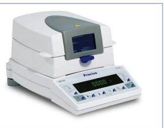
The moisture determination of liquid soap is essential to ensure a product of the highest quality. If the moisture content is too high or too low, this can result in a low quality product and wastage can occur.
