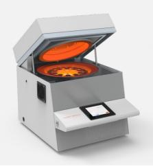
Moisture and ash are crucial analytical values in food samples and are often needed as calculation reference for other analytical parameters too. Furthermore ashing is part of the sample preparation for the analysis of individual elements in the mineral content. Moisture is a critical parameter for shelf life time of food and ash gives information on the salt content.
