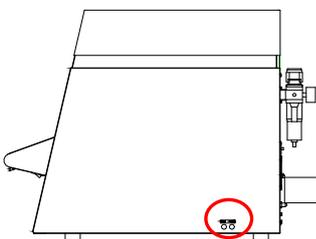
Press the „zero“ button
