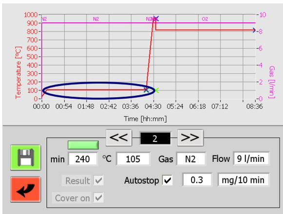
In Step 2 you can change the drying temperature and time. You are also able to add an autostop criteria. At the end of this step, the result is taken automatically and the lid is opening for adding the covers on the crucibles. **Don't put a cover on the reference crucible!**
