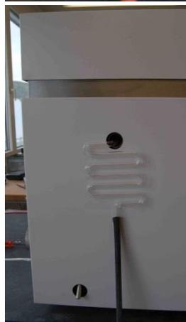
Insert the glass cooling coil through the hole on the left hand side of the prepASH into the centering lead.
