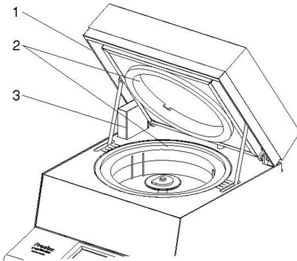
1 The circlip (1) prevents jamming when the lid is closed.
