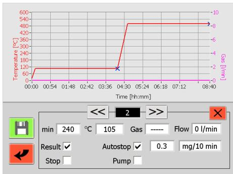
Choose the program step to be changed and overwrite the parameters needed.
