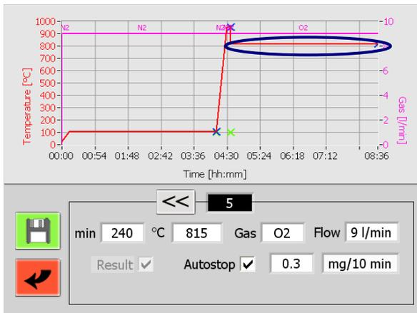
In step 5 you can change the ashing temperature and time. You are also able to set an autostop criteria. The result is taken automatically at the end of the step.
