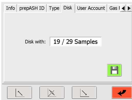
For the models prepASH229 and prepASH219 you can switch between the sample disks „19/29 Samples“ and „12 Samples“.
