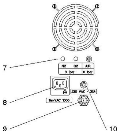
**7** The process gases can be fed in via the terminal connections (7) with hoses (outer Ø x thickness 4x0.75mm). The compressed air inlet (AIR) is connected to the maintenance unit in the factory.
