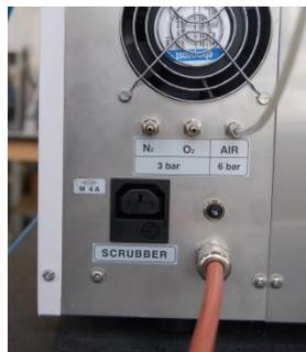
Connect the scrubber to the power outlet on the back side of the prepASH, see also chapter 2.4.2. Use the special Mains connection cable delivered with the scrubber connection set, 340-9002.
