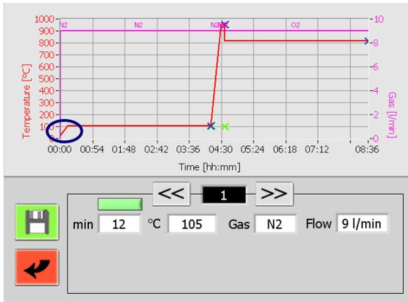
Step 1 is the ramp for the drying temperature. The ramp is limited to 50°C/min.
