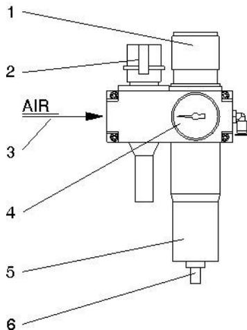
**1, 4** Use the controller (1) and the pressure gauge (4) to adjust the pressure in line with the pneumatic supply to the device.
