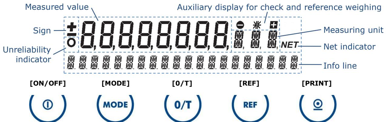
The measured value is stable as soon as the unit, e.g. "g", appears. The unreliability indicator lights up while the scale is recalculating the reference weight, for example, during counting, or when it is verified and in the warm-up phase.
