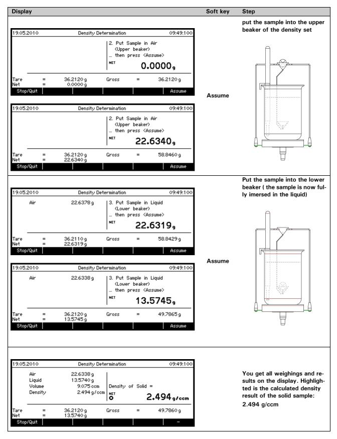
Density determination using below balance weighing Order number see Accessories of the respective series
