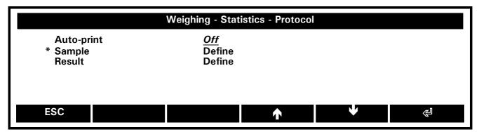
We reached the sublevel 3, as adverted by the headline which displays the entire path we have passed (Weighing - Statistics - Protocol).
