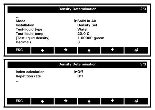
Installation: Density Set, Below Balance Weighing
