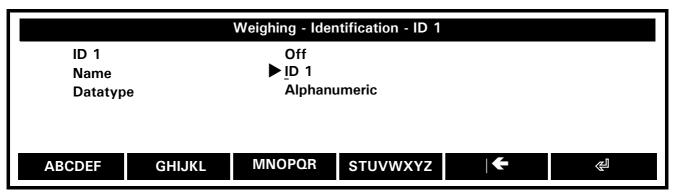
Doing text data entries, a wider range of additional soft key functions is available (observe the rotate symbol in the activity area and call them up by pressing **«ROTATE»**):
