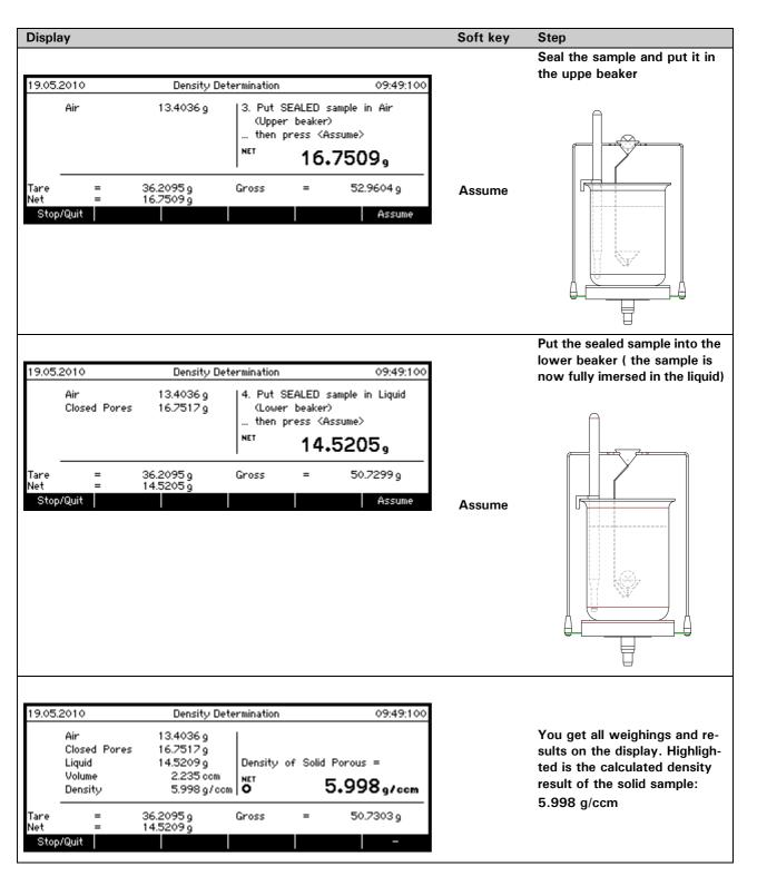
Density determination using a density determination set Order number see Accessories
