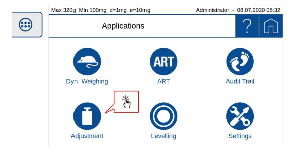
• Press **{Start}** ⇒ the balance automatically adjusts itself by meanings of the built-in self calibration system (SCS). When this is done it shows the message 'Adjustment done'.
