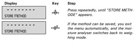
If the name has already been used for an existing method in the memory the method cannot be saved
