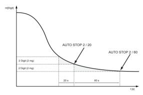
One digit is the smallest change in measurement that can be displayed by the moisture analyser.
