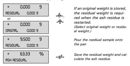
The ash residue is displayed until any key is pressed to print the ash residue protocol. Than the original and the residual weights are cleared.
