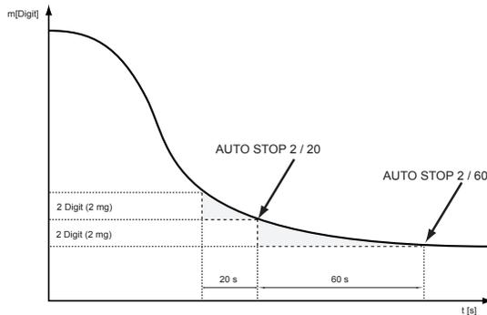
One digit is the smallest change in measurement that can be displayed by the moisture analyser.
