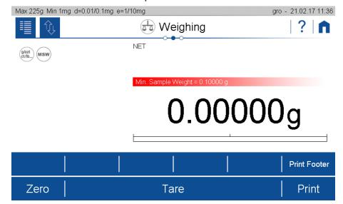
The required minimum weights should be determined on the basis of the QM specifications by means of the statistical analysis of certain series of measurements. The balance's own "Statistics" function could be used for this purpose, for example. It is used to perform and subsequently log the requisite series of measurements. Once the minimum weight(s) has/have been determined, it/they can be input into the balance. Up to three tare ranges can be defined with the corresponding minimum weights.
